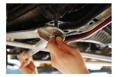
**Step 3:** Install new Allen head LCAB Bracket bolts with washers. Note: Over time, a lot of movement can occur in the uni-body, if the bracket bolts won't line up you can use a
